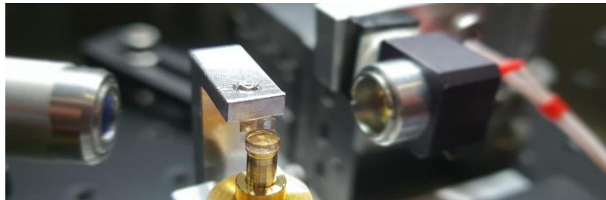
Diode: InP,  $\lambda=1535$  nm, spectrum width 10 nm (~50 lines),  $\Delta f \approx 17.6$  GHz,  $P = 200$  mW max
