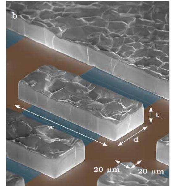
on-chip cooling of electrons with In refrigerant,
